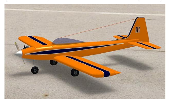
The retract mechanism makes for some weight and delicacy. The landing gear is prone to damage so the model should be flown from paved runways. The increased weight gives higher landing speed and the retracts should give higher flight speed. Unfortunately, the increase in flight speed is rather low.
