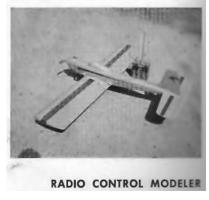
the leading edge got 0.25" backward and the trailing edge 0.75" forward. The center-of-gravity stayed at the same percentage of the chord length at the main spar. Obviously, just shortening the tail moment arm by 1.5" and leaving the tail areas unchanged gave about the same tail effectiveness.
