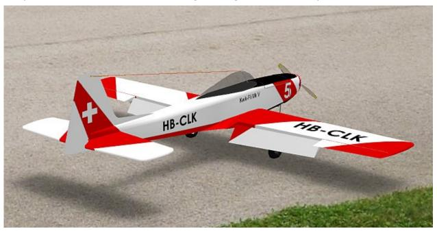
So models were equipped with speed brakes or flaps for glide angle control to facilitate spot landings. Unfortunately, in the newer versions of REFLEX XTR the coefficients for flaps and ailerons are the same, so it's not possible to give them different characteristics. Therefore, the "rocket" Kwik-Fli has no spoilers but normal flaps, which give lower approach speed due to more lift and a steeper approach due to much drag at 45 degrees deflection.
