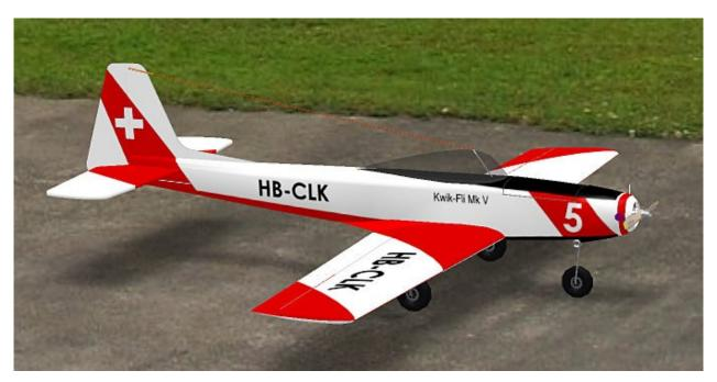
So there's one important modification left. The model has to be equipped with a thinner wing. The planform was left unchanged but different airfoils were assumed, instead of 20% to 15% from root to tip now 15% to 10%. As an average, the 12.4% thick Eppler E 168 was used to choose realistic coefficients. Though this is still not really thin, it gives somewhat lower drag and a really "ballistic" model, now even called "Mark V rocket" in REFLEX XTR.
