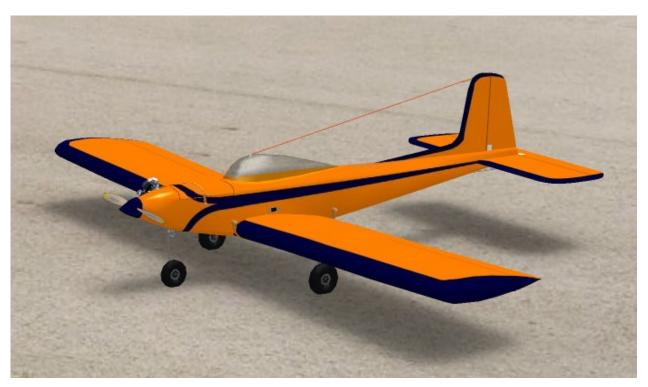
But soon this was taken for granted and Mark II with its smaller size and the same wing loading was appreciated for better authority in gusty wind. The better thrust/weight ratio obtained by using a .60 engine was appreciated as well, especially for competition where patterns flown faster look nicer or are easier to fly, respectively. Still Mark II doesn't fly really neat patterns and won't reliably spin or snap, not even the "crisp" version.
