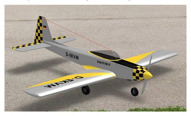
The model was an extreme lightweight to fly at slow speed. So some boxy shape and a tricycle landing gear didn't hurt but on the contrary contributed to the low weight. Much drag was good for constant slow flight speed, which is also why the wing airfoil was very thick (18%, or 20% to 15% tapered).
