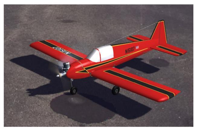
The simulator model has a Veco engine instead of the original's Enya 60 II, which was not available for modeling. The Enya is especially short so the Veco protrudes quite a bit, but that doesn't really matter.
