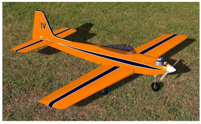
As usual and as for the basic design (see plan 5 pages above), Phil Kraft chose nice round numbers: 12" root chord and 9" tip chord giving a 0.75 taper ratio. The airfoil was modified as well by slimming a 20% thick root to a 15% thick tip. The 60" wingspan exclusive wingtips gave almost as much wing area as the 58x11" square wing. The ailerons got smaller, though, and require a bit more deflection.
