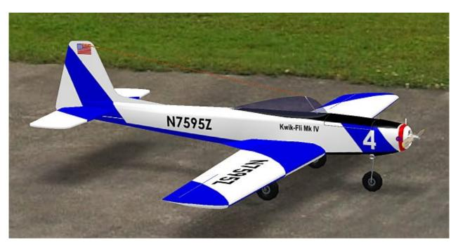
The first step was to put a Graupner/O.S. 49-PI rotary engine on it, which weighs only 395 g / 13.9 oz including muffler and mount. Of course, the Mark IV with retracts was chosen for it's low drag. The engine is able to take it to high speed because it may perform up to 2 hp at up to 20000 rpm if a hot fuel is used. It's low weight and small diameter are important as well. For more information about this engine see my article on Das Ugly Stik.
