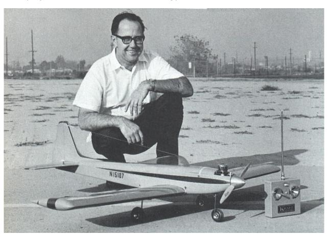
Ignore the nice guy on the picture; pay attention to the wing's leading edge. It seems to be especially sharpened, most likely for better spin and flick performance. It might just be a reflex but at least it's not a standard NACA 0019 noted for its blunt leading edge. The plan above shows a noticeably sharper leading edge. Anyway, the E 169 airfoil used for the simulator model shows an adequate stall behavior.
