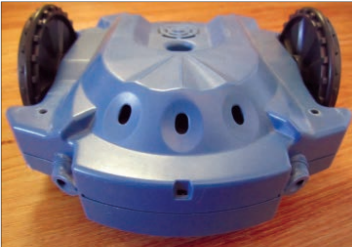
THE SCRIBBLER'S IR SENSORS ARE READY TO STARE DOWN SOME OBSTACLES.
