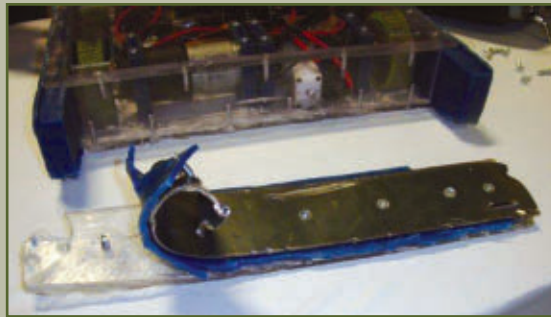
FIGURE 27. Steel bar peeled off 12 pound wedge bot Tough Nut by spinner bot Fiasco.
