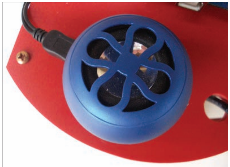
FIGURE 6. A self-contained capsule speaker incorporates its own amplifier, speaker element, and rechargeable battery.
