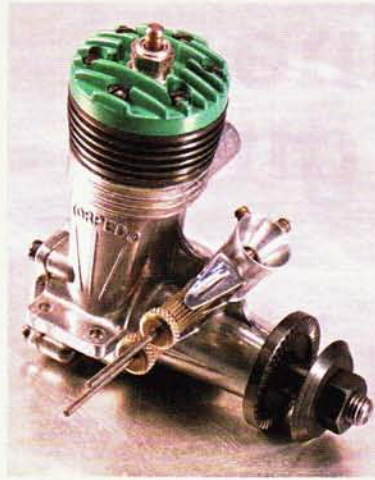
A vintage K&B “greenhead” .19 (1952) fitted with K&B’s early speed-control system. When operating from the low-speed needle valve, the engine was forced to run “4-stroking” rich. To avoid a sudden flameout, the first idle-bar glow plugs were employed.
