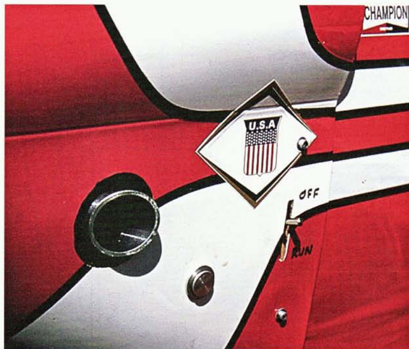
An engine kill switch is an important safety requirement for any IMAA flying event. Here, you see the toggle switch sticking out of a slot that I cut into my Pitts Special's engine cowl. The switch isn't anchored to the cowl itself; it is attached to the firewall with a plywood bracket.
