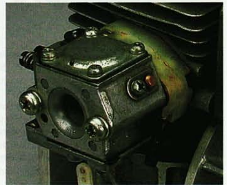
Not all carburetors have chokes; if yours doesn't have a mechanical choke, use your thumb to choke it while you rotate the prop to draw fuel into it.
