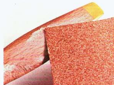
100-grit garnet abrasive paper works well for wooden propellers.
