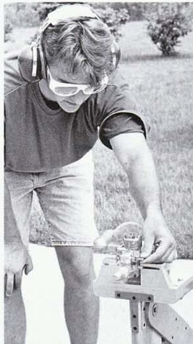
Always make engine adjustments from behind the prop.
