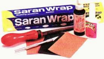
Materials needed to balance wooden and composite plastic propellers.
