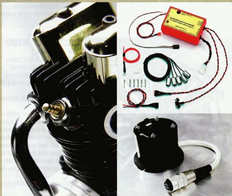
Top: the engine installation for Nick Ziroll's Stearman PT-17. Notice the multiple orange ignition-system wires that lead to each of the Robert R780's glow plugs. Below left: most radial engines are 4-stroke, glow-powered engines. Each cylinder head has one or more glow plugs. Below right: many radial-engine makers recommend the McDaniels onboard ignition system. It is available in several versions for single- and multi-cylinder engines up to 18 cylinders! Bottom right: the onboard ignition module from the RCS 215 engine. Note the robust wire connector for the gasoline-ignition engine.
