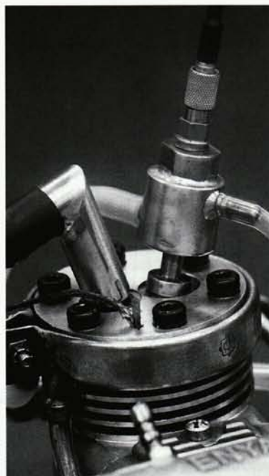
A water-cooled piezo-electric pressure transducer (right) has been mounted adjacent to the spark plug in a special cylinder head, which also contains a head temperature probe (foreground).
