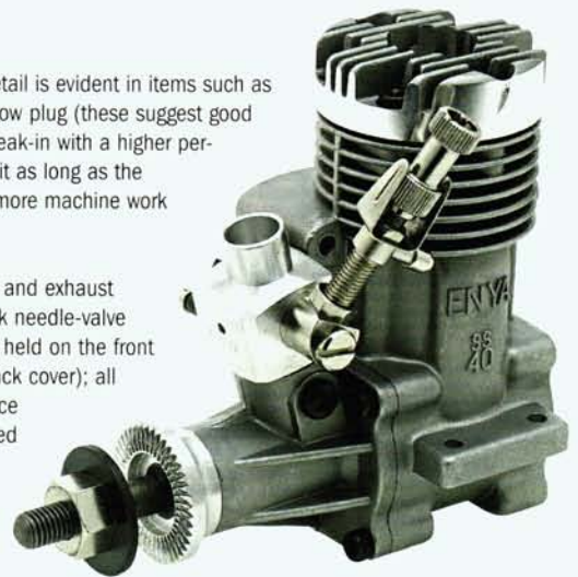
A plain-bearing Enya SS .40 with swept-back needle-valve; it has an iron piston and a steel cylinder, so it requires a longer break-in.
