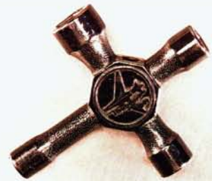
Using the correct glow-plug-removal tool minimizes the potential for damage to the plug and engine.
