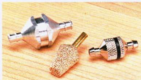
The large Du-Bro filter (left) is used on the bigger glow and gas engines. The sintered bronze filter from Du-Bro (center) can be used in the tank or in a fuel jug. The smaller Great Planes filter is perfect to use between the tank and the carburetor; it can be taken apart and cleaned.
