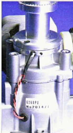
The B.H. Hanson 260 is a modified Zenoah G-26 with an electronic ignition system.
