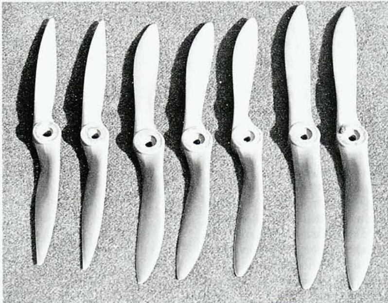
A family of propellers (APC) to be flown with a given engine/airplane combination. These have PLF numbers ranging from 363 to 605.
