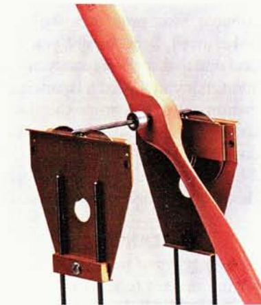
The High Point balancer with a 2-blade propeller. The heavy blade always hangs to the bottom.
