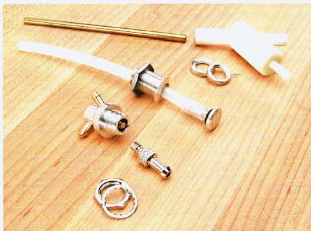
Above left: valves such as these from Sullivan (top) and Du-Bro (bottom) can be installed on the firewall. The R/C City fuel dot (center) is used in a 3-line fuel system, and it's foolproof. Above right: the Du-Bro spring clips come in sizes to accommodate small- and large-diameter fuel lines. Aerotrend makes neat little clamps that work well on Tygon fuel line. Trinity's nylon zip-ties are a quick and easy way to secure fuel lines.
