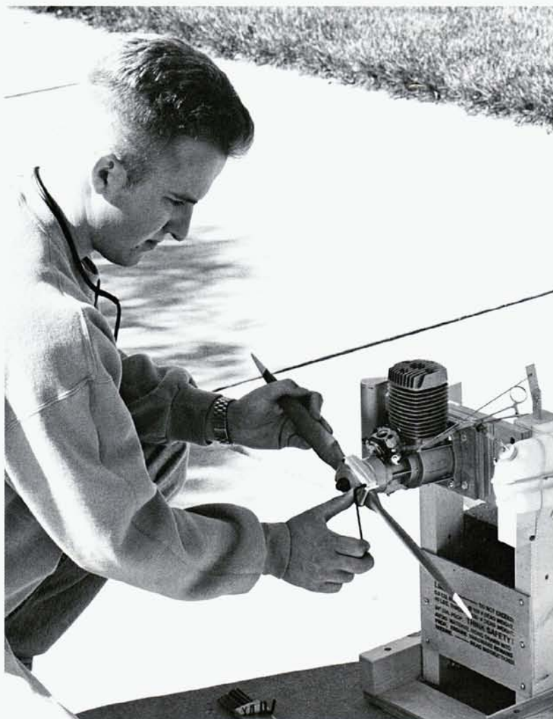
Preparing to start the large OPS 30cc 2-stroke engine for break-in on the large American Hobby Products test Stand, Gary Caruso tightens the hub on the two-piece APC break-in propeller.
