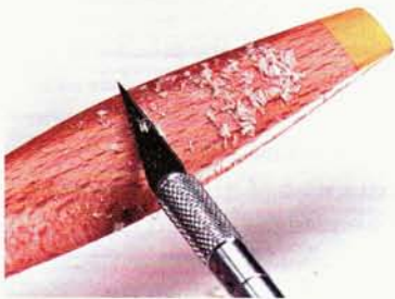
Use a hobby knife with a no. 11 blade to scrape the front side of the heavy blade to lighten it.
