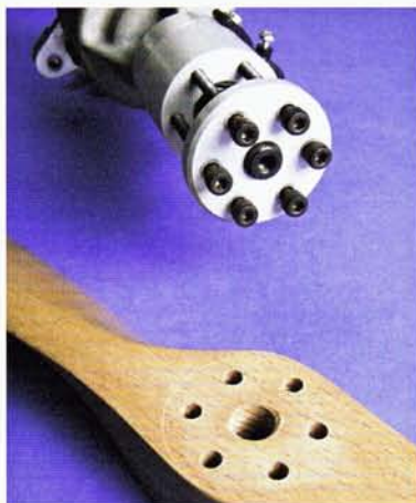
For multi-bolt prop hubs such as on this ZDZ 40 engine, use a drill press to drill the bolt holes. Be sure to position the holes so that there is a clear path of wood from tip to tip.
