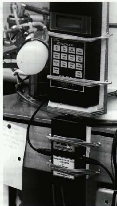
A tachometer frequency-to-voltage converter (bottom) was required for rpm data retrieval. The unit above the converter is a digital readout for exhaust gas temperature (used to set the needle valve to peak power).
