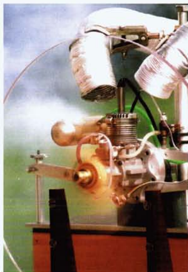
Dynamometer "load beams" are pitchless propellers that allow uniform increases in rpm from one size to the next; the author's beams are in \frac{3}{4} -inch increments from 2 to 10 inches.
