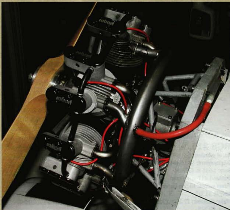
Top: the engine installation for Nick Ziroll's Stearman PT-17. Notice the multiple orange ignition-system wires that lead to each of the Robert R780's glow plugs. Below left: most radial engines are 4-stroke, glow-powered engines. Each cylinder head has one or more glow plugs. Below right: many radial-engine makers recommend the McDaniels onboard ignition system. It is available in several versions for single- and multi-cylinder engines up to 18 cylinders! Bottom right: the onboard ignition module from the RCS 215 engine. Note the robust wire connector for the gasoline-ignition engine.
