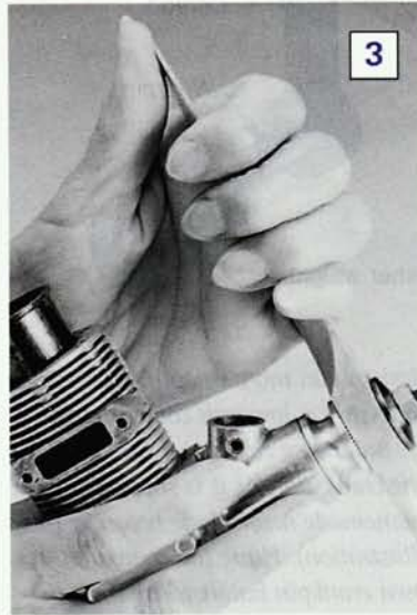
Photo 1. Place the copper glow-plug washer on top of the piston with its edge protruding into the sleeve's exhaust port. 2. Uniformly heat the upper crankcase with a low flame; hold the engine with an insulated glove (I use High Heat gloves). 3. The sleeve as it emerges from the crankcase.
