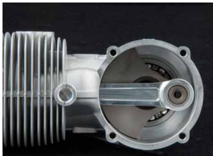
These two photos show the crankshaft and connecting rod at top-dead-center (TDC) and bottom-dead-center (BDC) to demonstrate how far things move inside the engine, at more than 100 times per second! The connecting rod is fully-machined aluminum with drawn-cup needle bearings pressed into each end.
