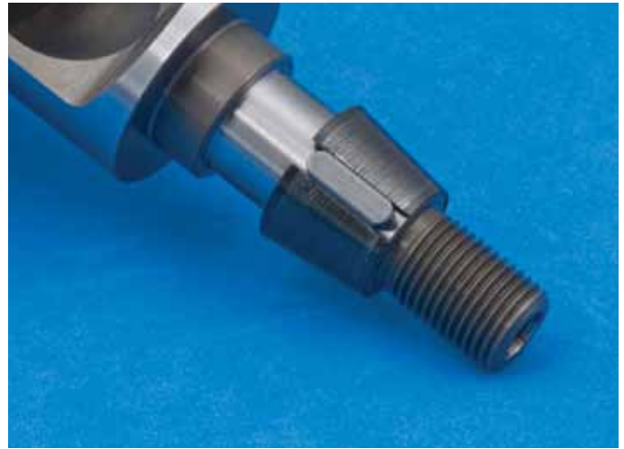
▲ O.S. applied a nice combination of tapered collet and a drive key to assure robust retention and rotational timing between the crankshaft and the propeller drive hub. Note how the large end-gap in the tapered collet fits around the key perfectly.
