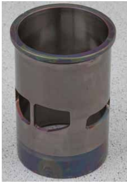
⤴ The steel cylinder sleeve features very neatly machined ports, and a super-fine honed finish in the cylinder bore. To the left is the large, bridged exhaust port, and to the right is the front transfer port.
