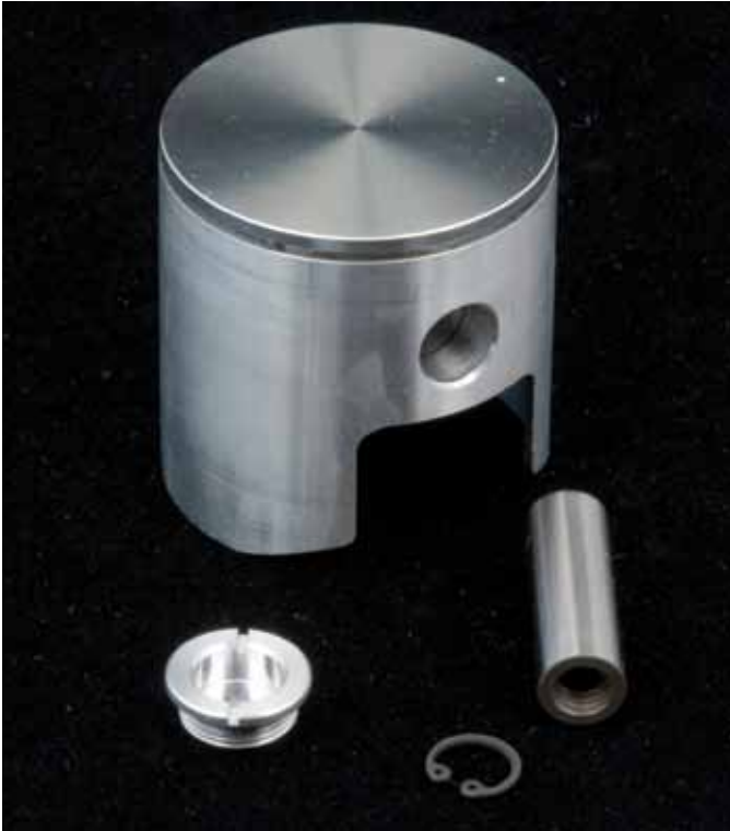
⤴ The piston is CNC-machine made from bar stock. It features a single, thin ring, large cutouts in the skirt to avoid blocking the entrance to the transfer ports, and the piston pin is placed high to allow the longest possible connecting rod length. The piston pin has internal threads to allow extraction through the access port in the rear transfer port casting.
