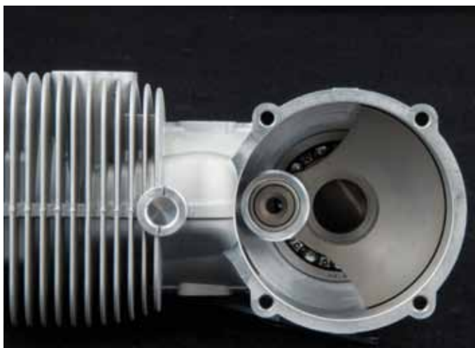
These two photos show the crankshaft and connecting rod at top-dead-center (TDC) and bottom-dead-center (BDC) to demonstrate how far things move inside the engine, at more than 100 times per second! The connecting rod is fully-machined aluminum with drawn-cup needle bearings pressed into each end.
