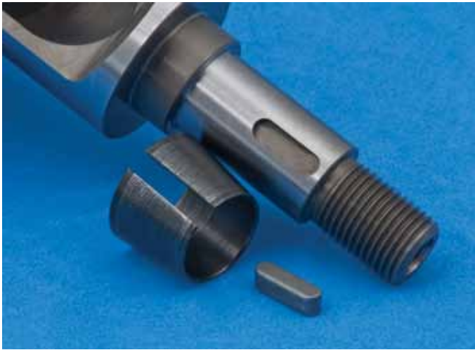
▲ O.S. applied a nice combination of tapered collet and a drive key to assure robust retention and rotational timing between the crankshaft and the propeller drive hub. Note how the large end-gap in the tapered collet fits around the key perfectly.
