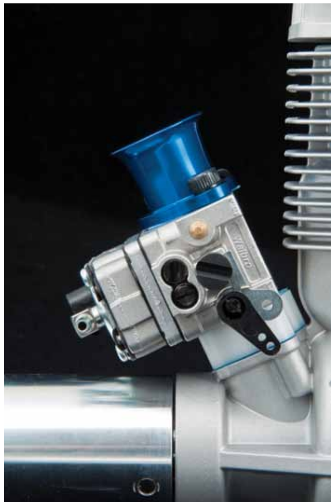
▲ The low-speed and high-speed needle valves, the idle-stop screw, and the throttle arm are all located on the left side of the carburetor. Note that they are recessed into the aluminum carburetor body.
