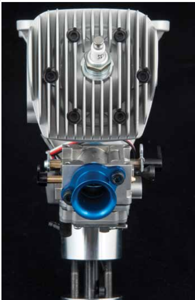
▲ This top view gives a good perspective on the cylinder head arrangement and attachment, using six M4 bolts for retention. The spark plug is angled rearward, and the exhaust side of the head has one more fin than the intake side.
