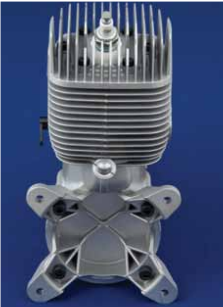
⤴ This view gives a good overall perspective of O.S.'s first gas engine offering. It follows their successful front-intake, rotary-valve configuration that has been used for years on most of their two-stroke glow engine lineup.
